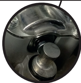
Position of unlocked motor : the pintle should be pressed
