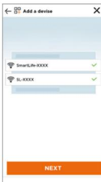
Connect the phone to the device's Wi-Fi access point.
