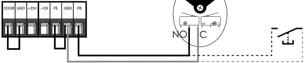
If the displays shows «E» then «4», the short-circuit between GND & DOOR is not correctly intalled.
