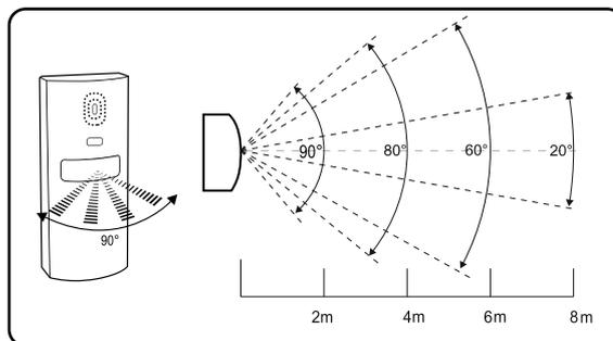
DÉTECTEUR D'OUVERTURE / OPENING SENSOR / SENSORE DI APERTURA
