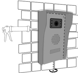
After installing and test, place a transparent acid free silicone seal at the top and on the sides of the door station (not at the bottom) to avoid any risk of infiltration.
