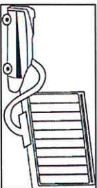
**NE JAMAIS UTILISER DE PRODUITS ABRASIFS OU BASE D'ACETONE QUI RISQUERAIENT DE DETERIORER LE REVETEMENT EPOXY.**
