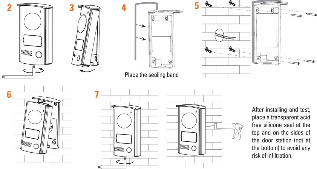
After installing and test, place a transparent acid free silicone seal at the top and on the sides of the door station (not at the bottom) to avoid any risk of infiltration.
