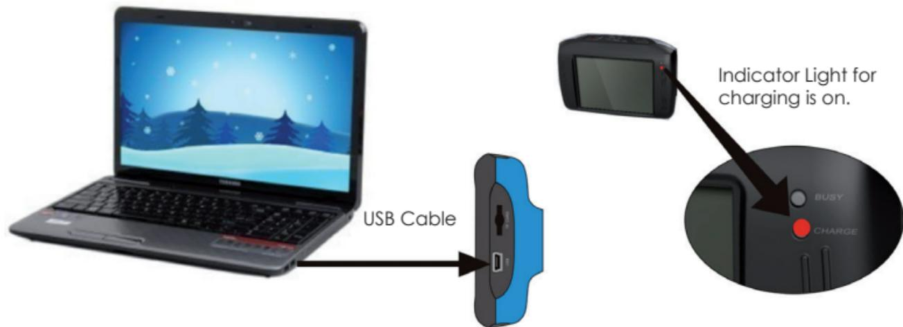
Connect the camera with computer for charging in the shutdown state. The indicator light for charging is on at this time and will be off after charging. In general, it can be fully charged after 2-4 hours.
