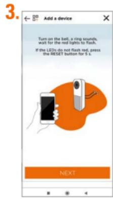
When the bell is flashing red, press next. If the bell is not flashing red, press the reset button for 5s.
