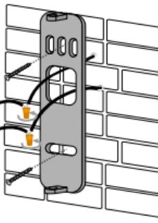
1- Install the wall support under a porch or a covered area is highly recommended.
