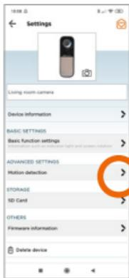
Press «Sensitivity» to manage the motion sensor. Higher is the «sensitivity», the more the camera will detect a motion.
