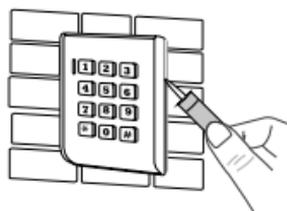
For a better seal, put silicone on the top and the 2 sides of the keyboard
